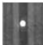
Fig. 1. Section of amplitude image of ILIT-measurement of CIGS-module with shunt in third cell. ( P_{in} = 30 \text{ W/m}^2 , Frequency = 1 Hz, Time = 33 min., open circuit conditions)
